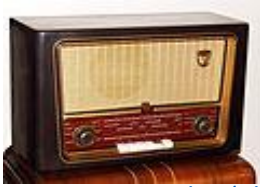
Vintage Norelco (Philips) Bakelite Table Radio With Push Buttons, Model BX548A, AM-FM-SW Bands, 8 Vacuum Tubes, Made In The Netherlands, Circa 1954 - 1955 (33175356006).jpg 2,884 × 2,184; 1.86 MB
