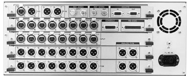
DMX-E3000 Rear Panel (Processor)
