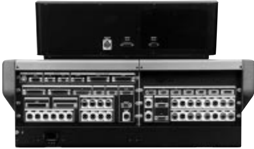
DMX-B4008A Rear Panel (Controller)
